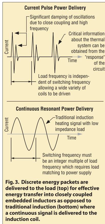
**Fig. 3. Discrete energy packets are delivered to the load (top) for effective energy transfer into closely coupled embedded inductors as opposed to traditional induction (bottom) where a continuous signal is delivered to the induction coil.**
