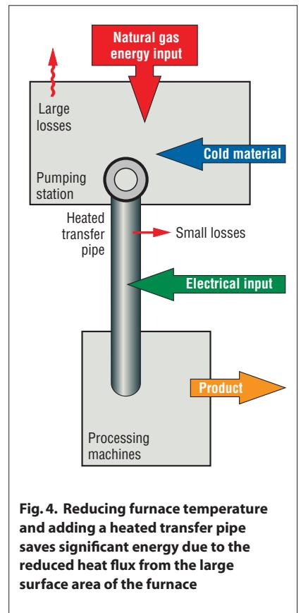
**Fig. 4. Reducing furnace temperature and adding a heated transfer pipe saves significant energy due to the reduced heat flux from the large surface area of the furnace**
